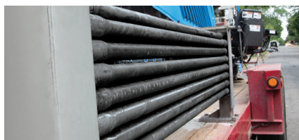
Drill rod capacity 61 metres optionally 76 metres
