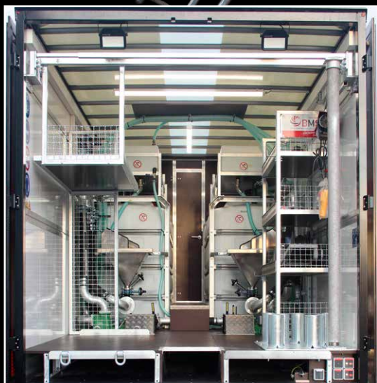
Rear view of the fixed superstructure of the BMS E2P mixing plant
